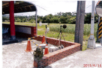
噪音振動監測情形 (104/6/14)
